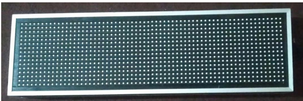
Gambar 4. Casing LED matrix P10
