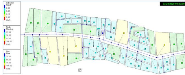
Gambar 6. Hasil Simulasi SWMM Kondisi (a) eksisting, (b) Vegetative Swale , dan (c) Permeable Pavement
