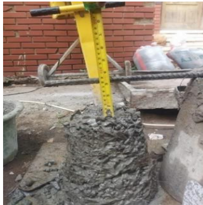
Gambar 2. Uji Slump Beton
