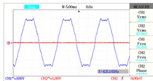
Gambar. 6. Generator Sinkron Tanpa Beban
