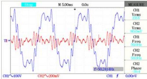
Gambar. 7. Generator Sinkron Dengan Beban Kapasitor 30uF
