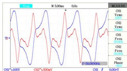
Gambar. 12. Generator Sinkron Dengan Beban Kapasitor 90uF
