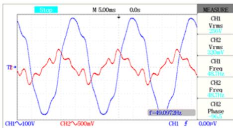
Gambar. 9. Generator Sinkron Dengan Beban Kapasitor 60uF
