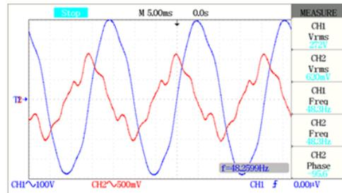
Gambar. 11. Generator Sinkron Dengan Beban Kapasitor 90uF
