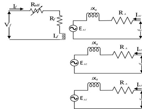
Gambar. 1. Rangkaian Ekivalen Generator Sinkron
