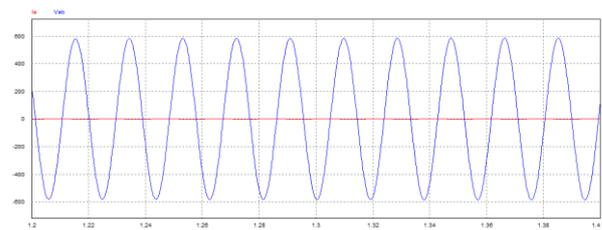
Gambar. 5. Simulasi Generator Sinkron Tanpa Beban
