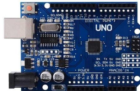
Gambar 2. Board Arduino Uno R3.
