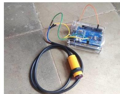
Gambar 13. Rangkaian sensor proximity infrared.
