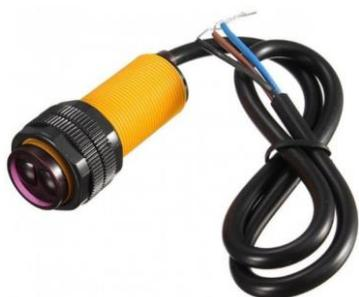
Gambar 5. Sensor Proximity Infrared.
