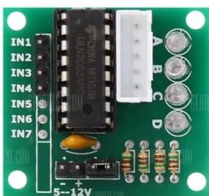
Gambar 4. Driver Motor ULN2003.
