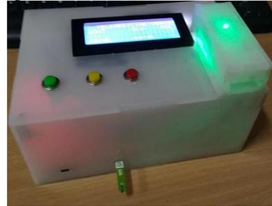
Gambar 3. *Device Prototype Telemedicine* Asam Urat
