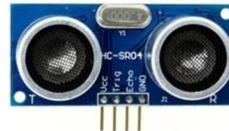
Gambar 2. Sensor Ultrasonic HC-SR04.
