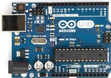
Gambar 1. Arduino Uno DIP.
