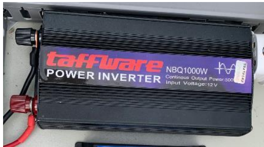
Gambar 5. Inverter Continuous Output 500W
