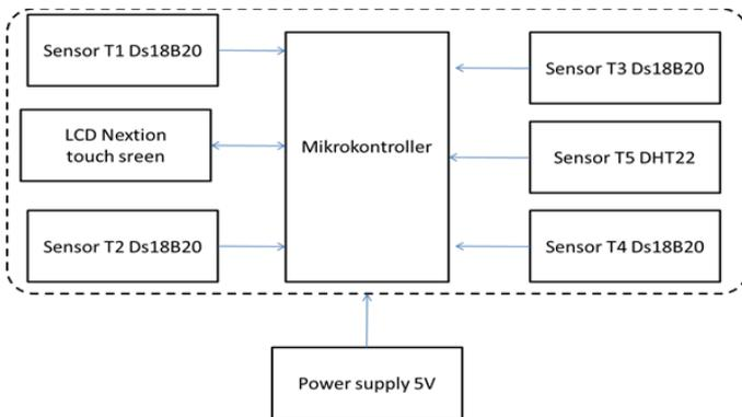
Gambar 1. Blok diagram INCU Analyzer berbasis Arduino UNO
