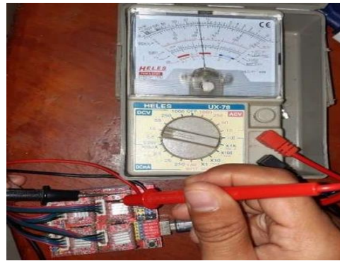
Gambar 34. Pengukuran Driver Motor A4988 Sumbu Z
