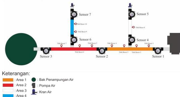
Gambar 6. Desain *Plotting* Area Kebocoran Pipa
