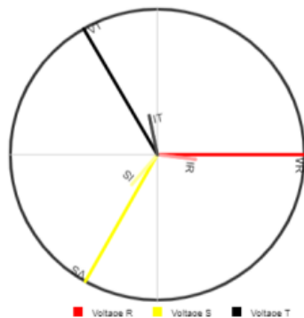
Gambar 13. Diagram Phasor Hasil Penarikan Data BUSTAMIN Melalui Sistem AMR
